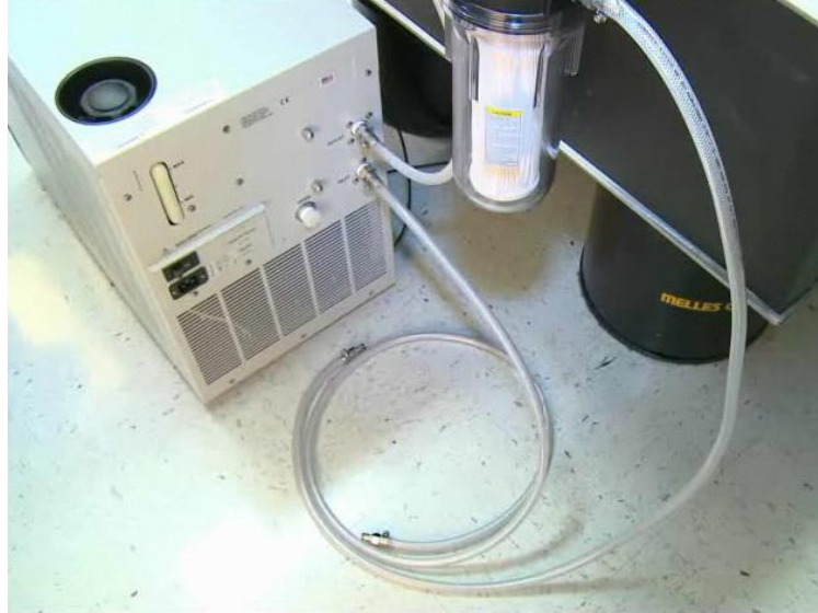
Figure 4-4 Chiller Assembled with Coolant Hoses and Filter
