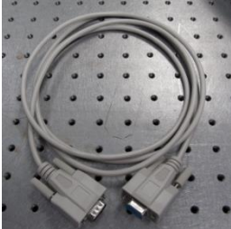
Chiller to Controller Cable
